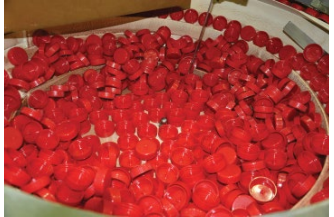
Fig 3.2. Fully automatic Specimen Container production line - Cap feeding.
