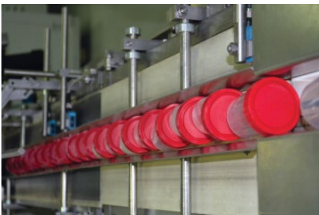
Fig 3.5. Fully automatic Specimen Container production line - Assembled product.
