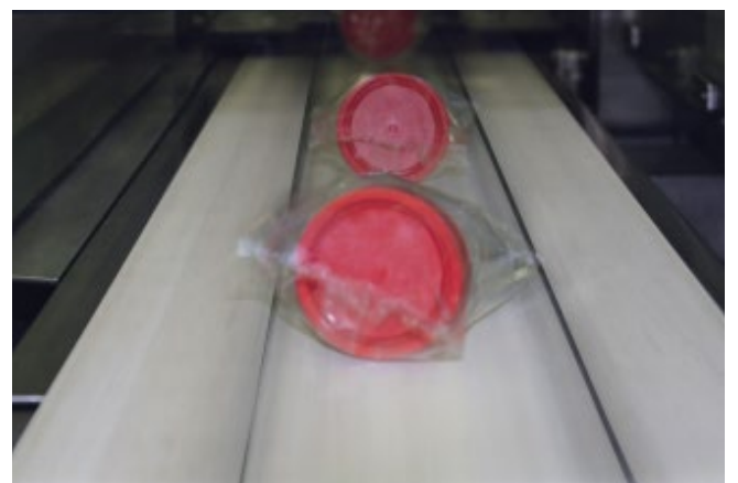
Fig 3.6. Fully automatic Specimen Container production line - Product packaging.
