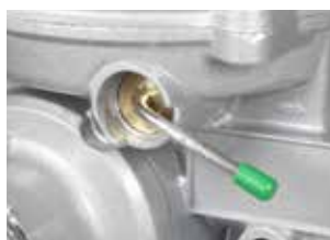
Reset excess flow with lever
