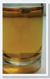
Place disc in a small volume of a suitable broth medium such as brain-heart infusion
