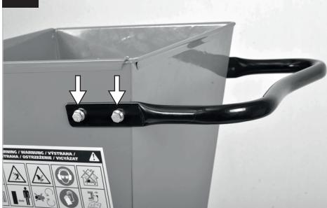
**EN** Attach the filling channel handle. Pay attention to the chamfering of the flat parts of the handle while attaching it. The chamfer must be in the same direction as the chamfer of the filling channel.
