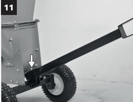
**EN** Attach the drawbar if necessary.
