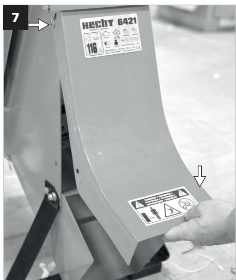
**EN** Remove the two wing nuts on the sides of the removal channel in the area below the engine. Place the removal channel cover onto the screws. At the bottom, tighten it with two M8 screws. Install the wing nuts and tighten the cover.
