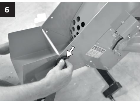
**EN** Before attaching the wheels, first install the front support. Lift the machine on the other side (the removal channel side). First, remove the short M8 screws and the long screw on which the spacer is mounted. Then align the bottom plate with the screw holes. Attach the front support from the outside so that the slanting cut on it is outward. Put all three screws where they were pre-assembled and tighten firmly.
