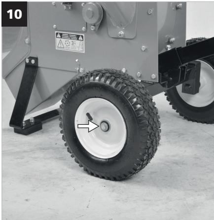
**EN** Remove the wheel screws and add the wheels (by longer placement of the centre inwards, the valve outward).
