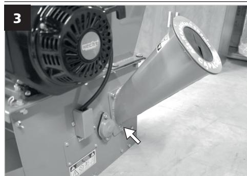
**EN** Attach the side filling channel first. Tighten firmly.
