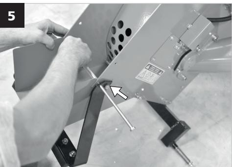
**EN** Lift the machine body on the filling channel side and attach the transport wheel axle by the four M8 screws. Pay attention to possible turning. The axle is attached so that the slanting drawbar attachment is higher on the side forward (from the machine).
