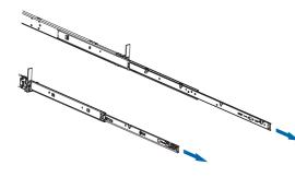
4 Align the rail standoffs on each side of the system and lower them into the slots on the rail. Put the system downward until all the rail standoffs are seated in the slots.
