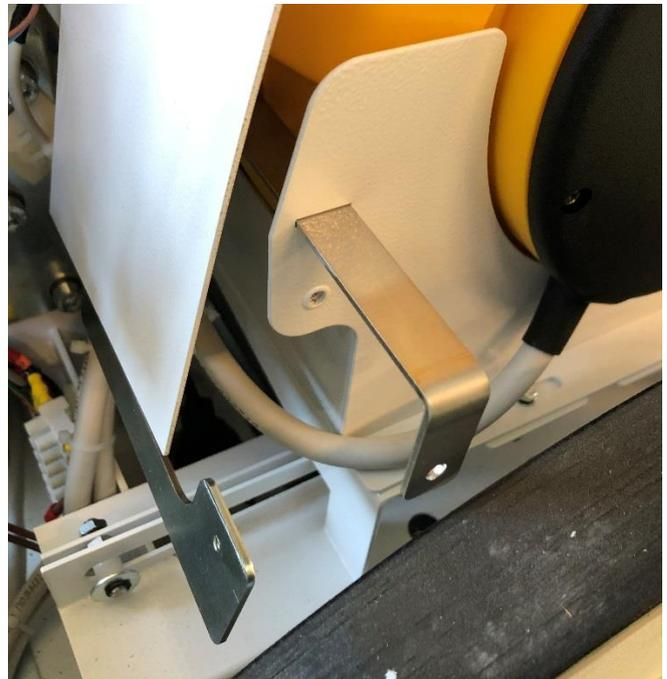
Remove the cable reel from its seat, cut the cable ties that block the cable out of the wiring
