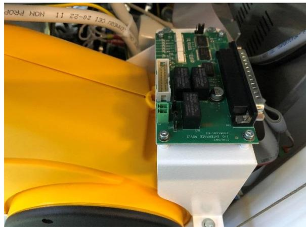
Remove the cover on which the I / O board is attached to gain access to the cable reel, unscrewing the three M4x12 bolts using a 7 mm key
