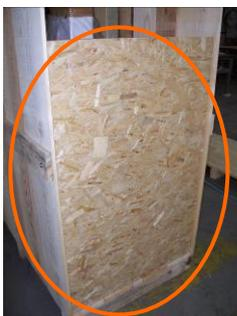
2. Remove the platform and the beams, removing the screws visible from the outside of the box
