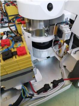
Last operation, carefully position the battery pack on the top cover of the UPS.
