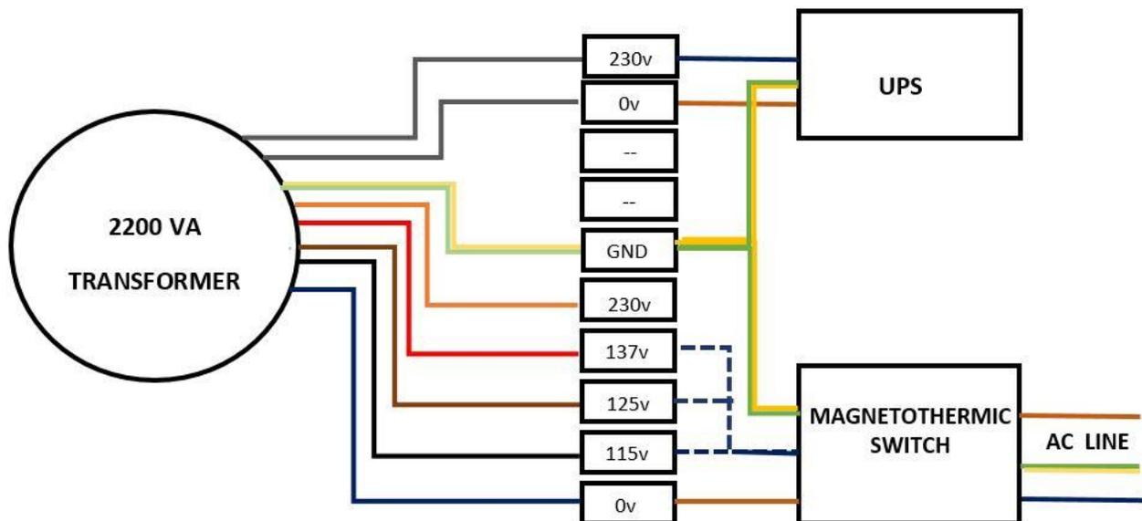
The wiring of the isolation transformer for the 115 AC line is very similar to the other; The only difference is the connection of the input wires to the transformer.
