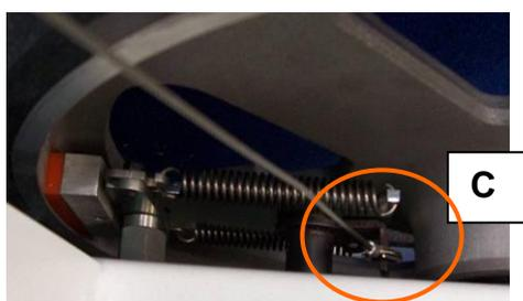
**IMPORTANT:** For have a good functionality of the brake is necessary to have a little tension of the iron cord.
