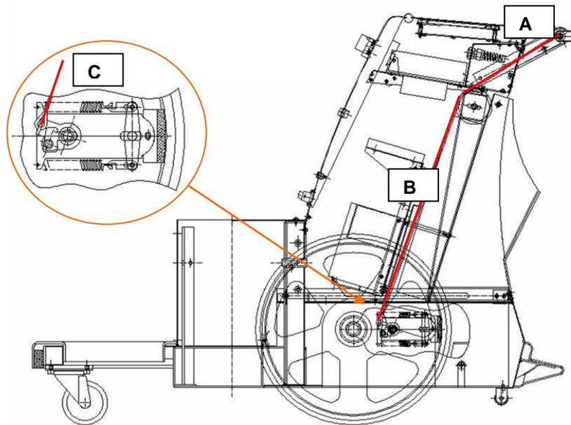
For replace the brake iron cord is necessary to remove the cover of the unit. After the remove of the cover for change the iron cord of the brake is necessary:
