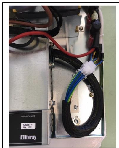
At this point, the electrical connections between the batteries and the rest of the system are completely removed and it is possible to disassemble the batteries.
