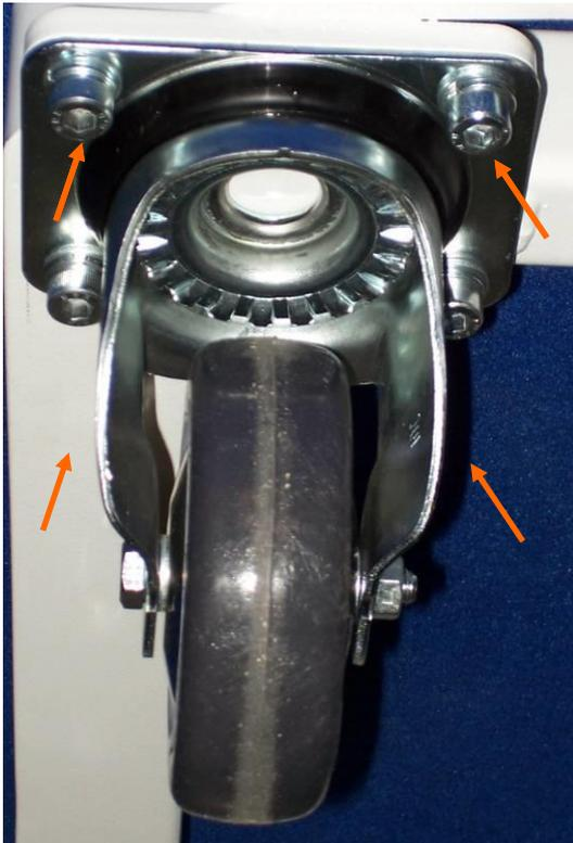
To replace the front wheels, loose the 4 screws indicated whit the arrows.
