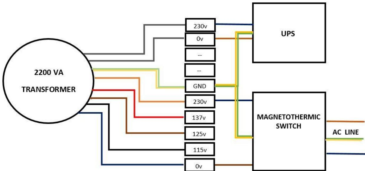
General scheme of the wiring of the isolation transformer for 110/115V devices.
