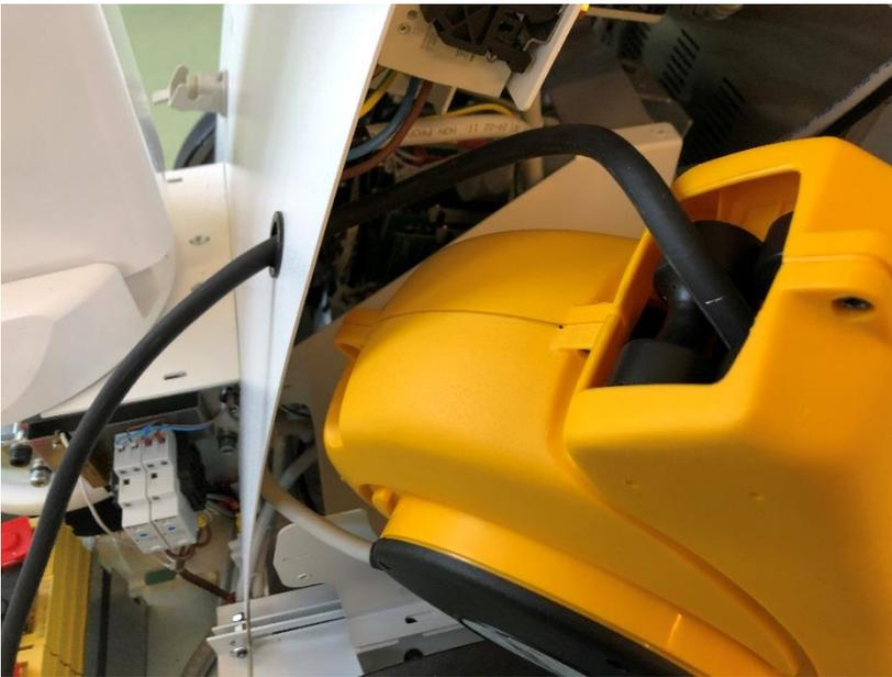
Remove the magneto-thermal switch from its seat, connect the wiring coming from the cable reel.
