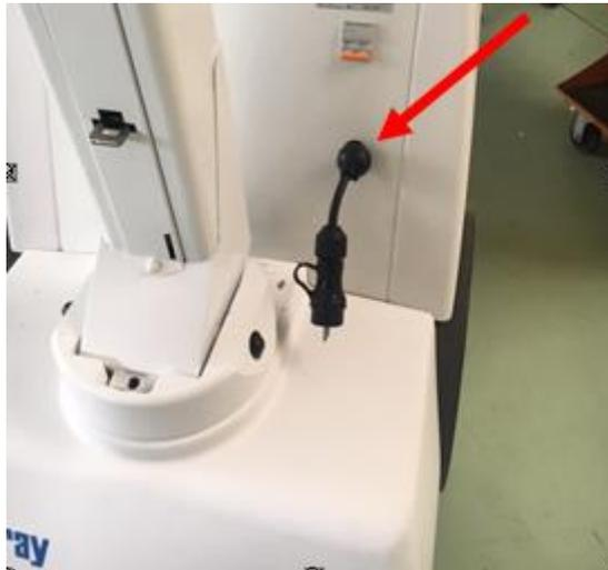
To store the power cable, unplug it from the mains, pull it slightly to release it and gently accompany it until the wire is completely retracted.
