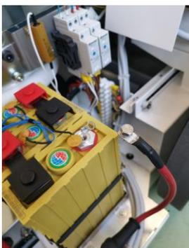
First operation, remove the positive conductor from the last cell, it will be easier to move the battery pack.
