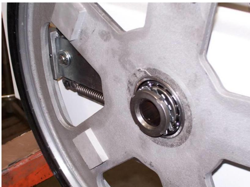
To replace or remove the rear wheels is necessary remove the wheels cover and loose the iron ring indicated whit red arrow.
