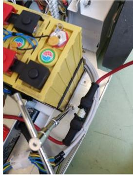
Then, remove the two fixing screws that secure the battery pack to the metal floor
