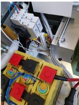
When this operation is necessary, since the terminals are positioned behind one of the two battery packs, the operator must remove it to have the possibility of working better.
