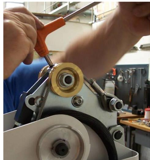
**IMPORTANT:** *If after have tight to maximum tension the nut, the arm do not take the right position to balance IS NECESSARY TO REPLACE THE GAS SPRIG KIT.*
