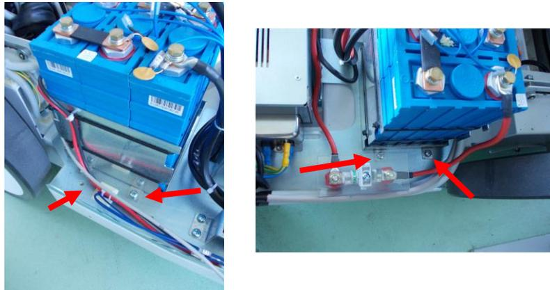
Follow the reverse procedure to install the new batteries. Due to the two battery packs are not equal in size, respect the positions.
