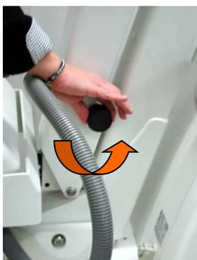
Check that the hook of the arm takes the arm in block position to the column the loose hooking is the cause of deterioration of the components, is necessary to replace the hooking system.
