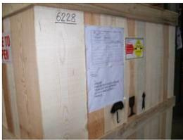
A shockwatch label and the handling and destination instructions are applied on the outside of the box.
