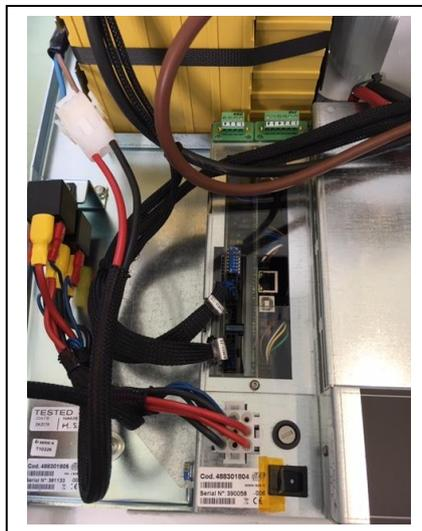
Disconnect the two connectors on one side of the UPS holder (see the figure below).
