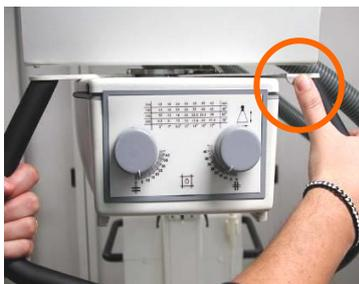
The collimator can rotate +/- 90° around the axis of the x-ray beam. The collimator’s rotation travel is limited by a mechanical stopper.
