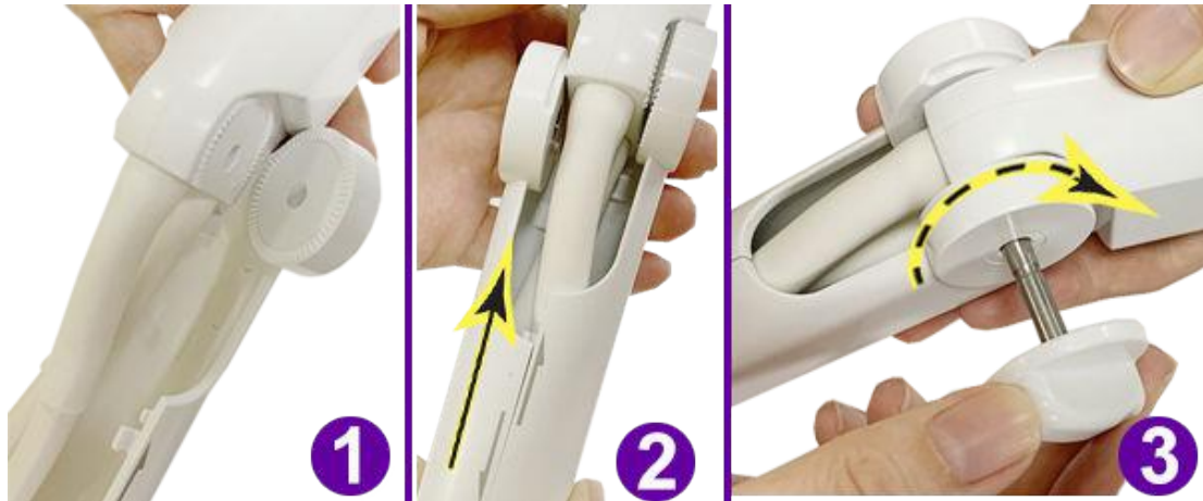
Figure 5-18 Reassemble the probe
