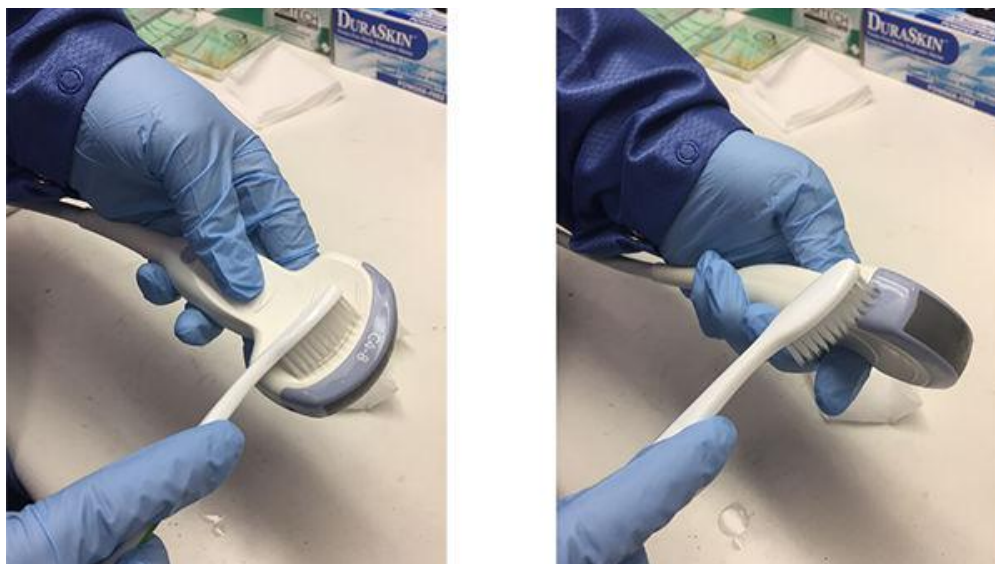
Figure 5-5 Cleaning the probe using a brush
