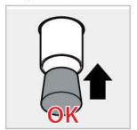
If the BAKERTOP MIND.Maps™ oven cannot be permanently connected to a drainage system, the terminal must be sealed with the conical plug supplied in the starter kit. When the terminal is blocked, DO NOT use the wash programs or wash the cavity with large quantities of water. Risk of flooding.
