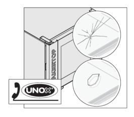
If the appliance glass is chipped or damaged, it must be replaced immediately. Please contact an authorised support service centre. Do not use the oven. Risk of exploding glass.
