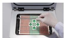
4. Load baskets and start Load one or two baskets, then start processing.
