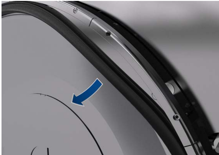
Figure 142: Pulling out the door seal
