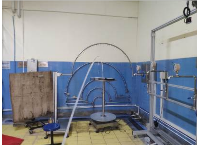
Photo 4 -- During the test of IPX5
