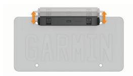
4 Insert the license plate screws through the top of the license plate and mount, and into the license plate mounting holes on your vehicle.
