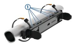
2 Tighten the zip ties to ensure the mount does not move during use.
