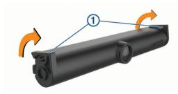
2 Insert a AA battery into each end of the camera, with the positive pole facing outward.
