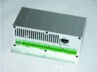
Field Multimedia Converter provided with 5 RS 485 ports, 1 Ethernet port and 1 RS 232 port in aluminium case.
