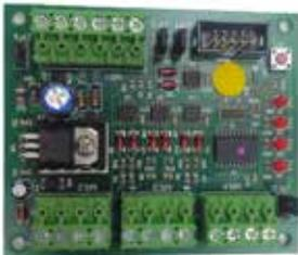
Field Bus repeater/converter for Serial Line RS-485-1 Input / 3 Output - naked version.
