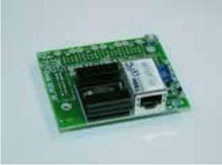
"Add on" card for IB-Hub Upgrade. Includes ETHERNET port.
