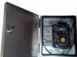
Fiber optic Controller (1 PCB) including IP65 box, 1 zone, up to 1km. The analyzer evaluates difference between transmitted and received light through optophonic technology. The signal, duly filtered out and processed, generates cut or climbing alarm. The controller unit is provided with stainless IP65 box and power supply.
