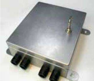
Fiber optic Controller (2PCB) including IP65 box, 2 zones, up to 2km. The analyzer evaluates difference between transmitted and received light through optophonic technology. The signal, duly filtered out and processed, generates cut or climbing alarm. The controller unit is provided with stainless IP65 box and power supply.
