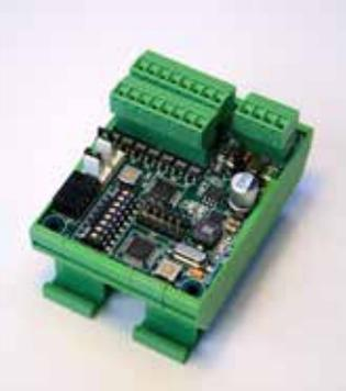
Master board with 8 dry contacts (4 overall status + 4 zones). Expandable up to 20 zone dry contacts (+ 4 overall status). Master board with 8 dry contacts (4 overall status + 4 zones) via RS-485 up to 1,2 km. Note: To reach the maximum expansion of 20 dry contacts (20 zones) it's necessary to add 2 SIOUX-CARD-8S.
