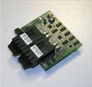
Additional tool for integration on IB-HUB with 2 Single-Mode fibre optic ports.
