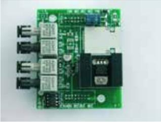
Additional tool for integration on IB-HUB with 2 Multi-Mode fibre optic ports.
