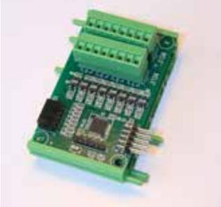
Slave relay expansion board with 8 relays (requires a SIOUX-CARD-8M)
