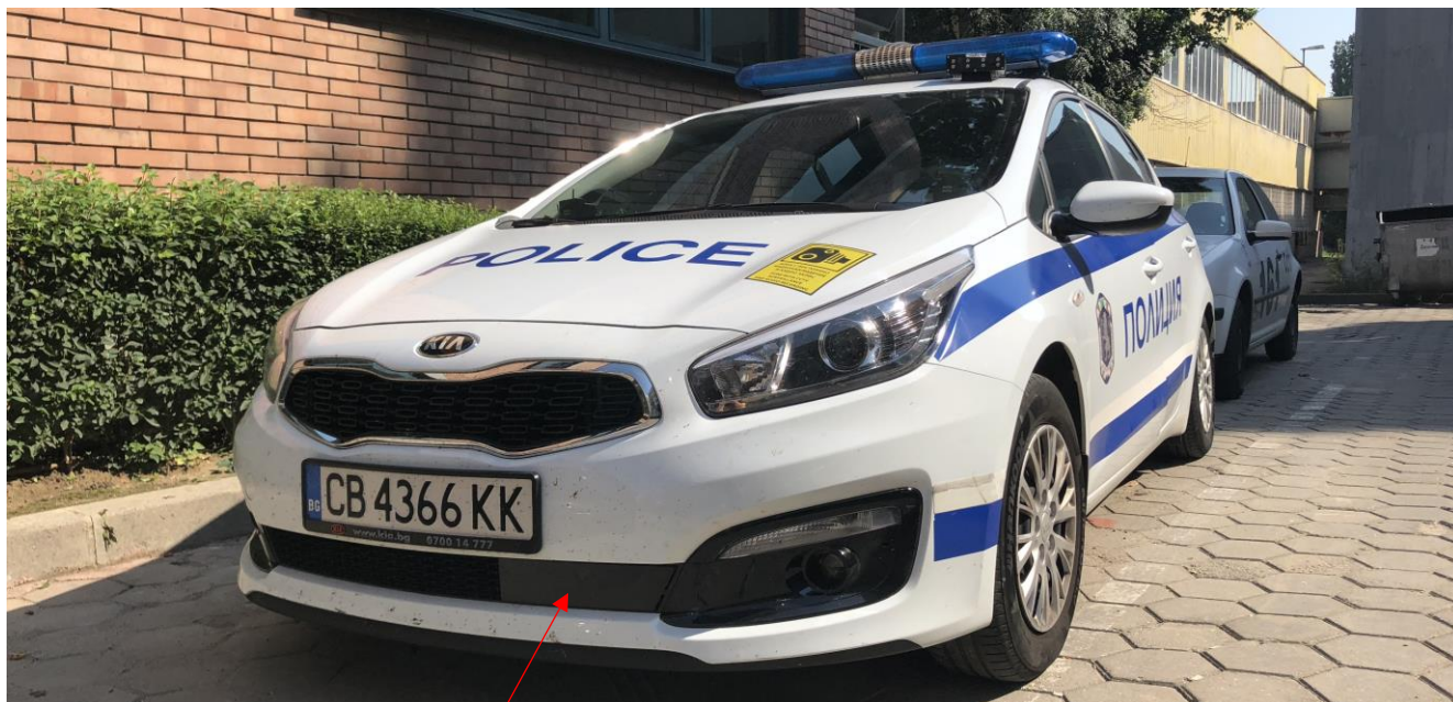
Radar antenna, hidden in the front bumper
