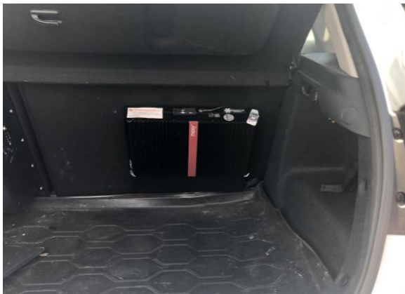
Installation of the computer (Q*BOX) in the trunk of the car
