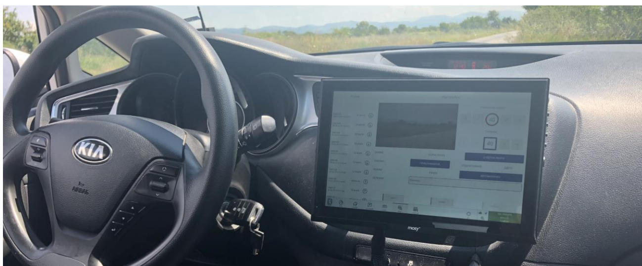
Touch Screen installed on the dashboard
