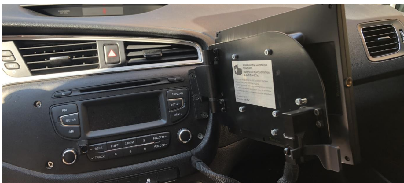
Discrete but robust fixed mounting. Possibility to tilt the Touch Screen.
