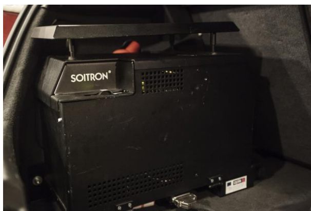
Complex HW covered in a dedicated box in the trunk of the car
