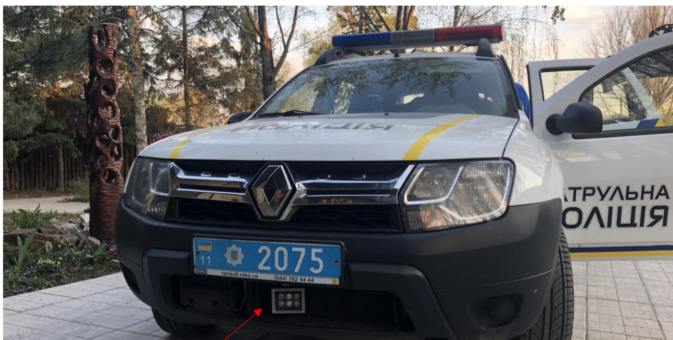
Installation of the IR light in the bumper (the picture is uncovered – without the grill)
