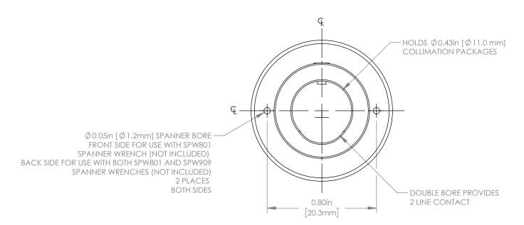
THORLARS DRAWING PROJECTION  $\bigoplus$ NAME DATE Ø11.0mm COLLIMATION TO SM1 ADAPTER CG 28/AUG/14 REDRAWN 28/OCT/14 MATERIAL APPROVAL PG REV N/A D COPYRIGHT © 2014 BY THORLABS APPROX WEIGHT ITEM # VALUES IN PARENTHESIS ARE CALCULATED 9.1 g AD11F AND MAY CONTAIN ROUNDOFF ERRORS
