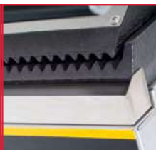
Grease and debris collection gutter
