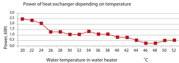
This graph represents the dependence of the power of the heat exchanger on the water temperature in the water heater. The data were obtained under the following conditions:
