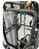
low pressure switches – FRP or stainless steel membrane covers – TFC type RO membranes – High pressure pump – Pressure setting valve – Dual water connection designed for RUMED / CSSD use.
