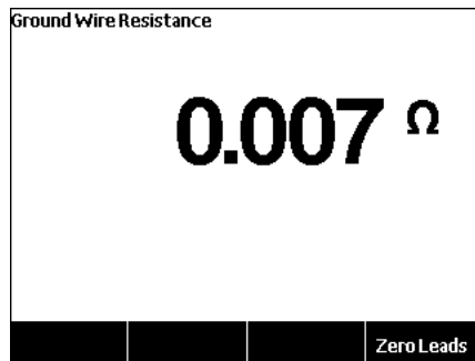
Figure 11. DUT Ground Resistance Measurement
