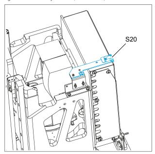
4. In the service screen for **End Limit Switch Check**, the low display for Table Lift and Table Tilt is set to OK (→ Pfeil/Fig. 64 Page 119). This means that the S20 tilt switch is activated.
