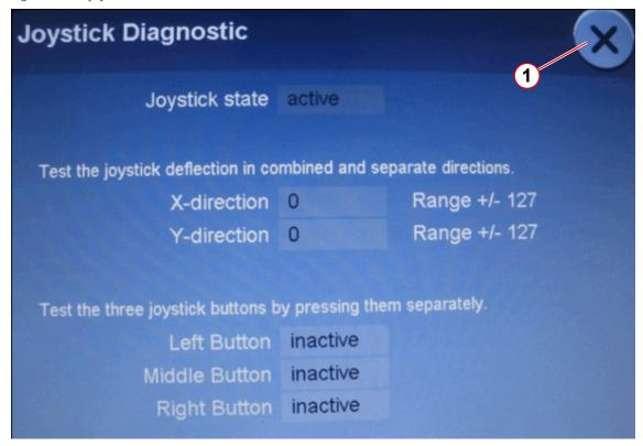
7. Once all functions have been tested, end the test at the ECC (> 1/Fig. 16 Page 32).
