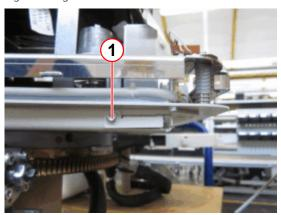
(1) Tighten the screw (ISO4762, M3x6)
