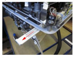
4. Replace the old air filter pad with the new air filter pad.
