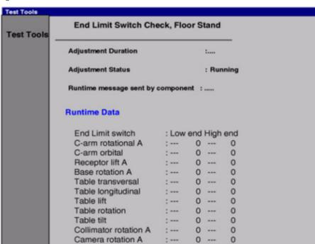
Fig. 49: End Limit Switch Check, Floor Stand
