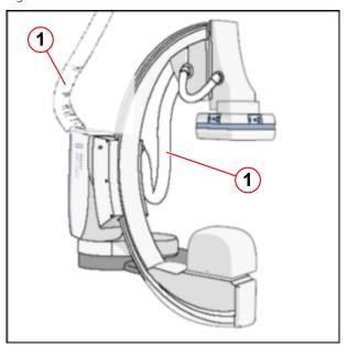
1. Check the cables and corrugated hoses for damage (→ 1/Fig. 55 Page 104).
