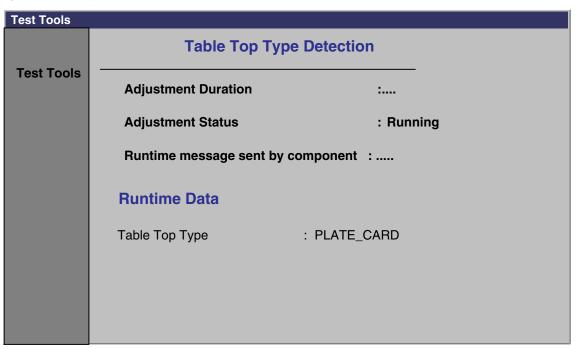
7. Insert the tabletops that are configured and check whether these are correctly sensed.
