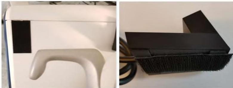
**Figure 3-21** Placement of Velcro tape
