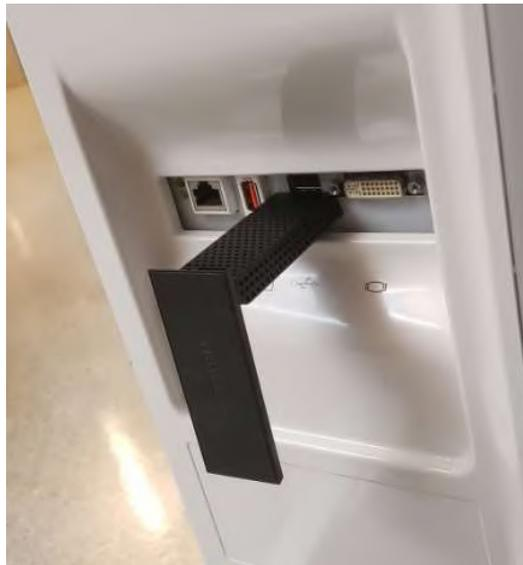
**Figure 3-23 Connecting wireless network adapter to rear USB-port**
