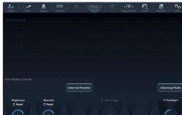
Figure 6-1 LCD adjustment utility
