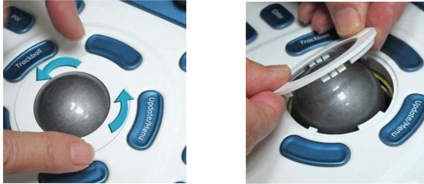
Figure 4-12 Removing Top Locking Plate and Rubber Dust Filter Ring
