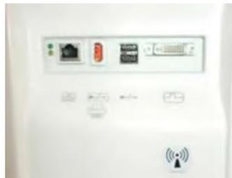
**Figure 3-24 Placement of wireless network Label on Vivid S60N/Vivid S70N**
