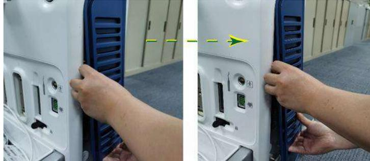
**Figure 8-3 Removing the Air Inlet (Left Side) Cover**
