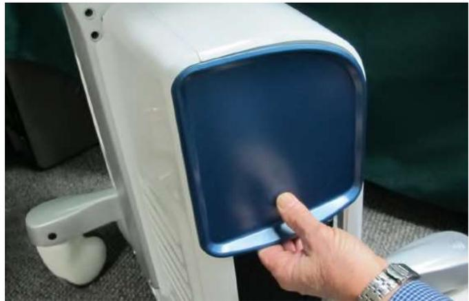
Figure 8-8 Removing the Blank Cover
