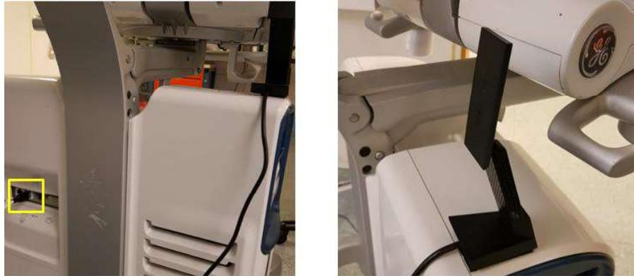
**Figure 3-22 Placement/Connection wireless network adapter**
