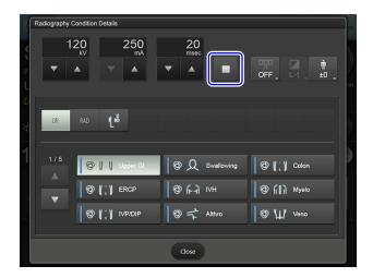
Press [Close] when the settings are completed. The [Radiography Condition Details] screen closes.
