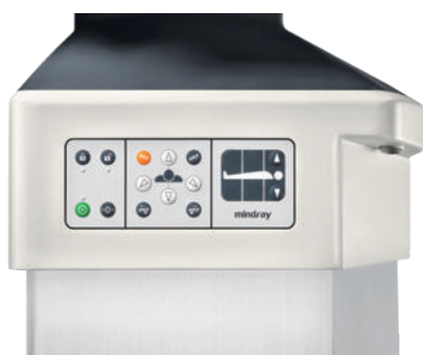
Override panel (Backup control panel)
