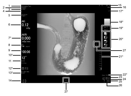
The display specification for items with "\*" changes depending on the detector type.
