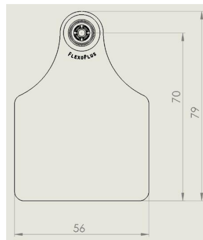
FlexoPlus D, mother part, dimensions
