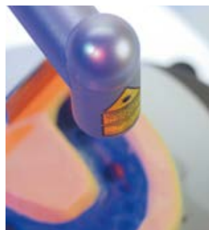
Laser beam for easy drill positioning
