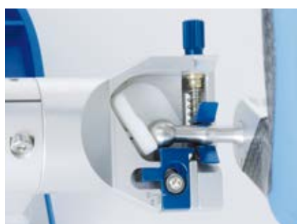
A) Artex®CR condyle in centric position viewed from below
