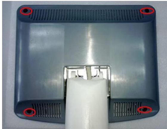
Figure 6-6 Diagram for Dismounting of Rear Cover of Display
