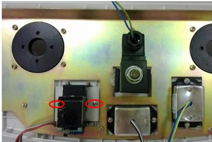
Figure 6-19 Diagram for Dismounting of DPM
