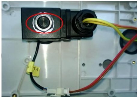
Figure 6-15 Diagram for Dismounting of Valve
