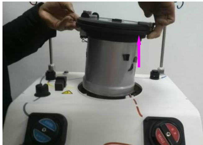
Figure 6-18 Diagram for Dismounting of Centrifuge Assembly III
