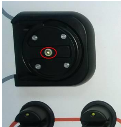
Figure 6-20 Diagram for Dismounting of Pump Assembly I
