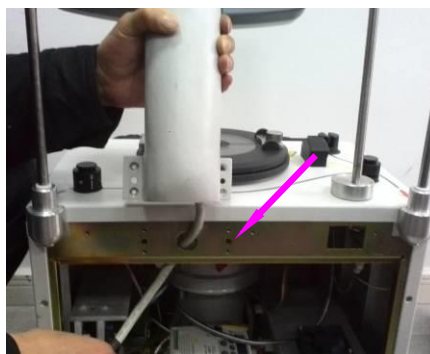
Figure 3-2 Communication Cable Threading
