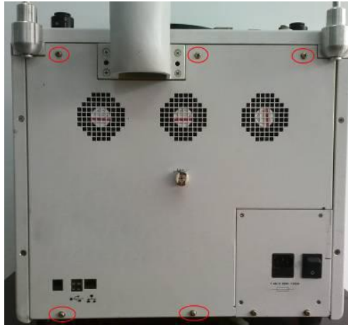
Figure 6-4 Diagram for Dismounting of Rear Cover of Host
