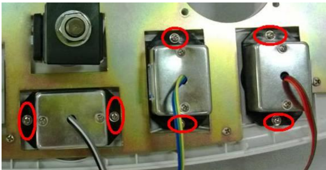
Figure 6-14 Diagram for Dismounting of Air Detector Modules
