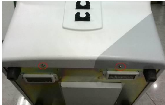
Figure 6-3 Diagram for Dismounting of Front Cover of Host
