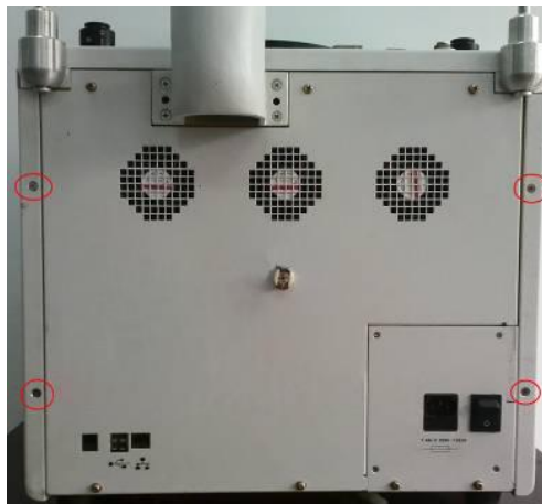
Figure 6-5 Diagram for Dismounting of Left cover and Right cover of the Host
