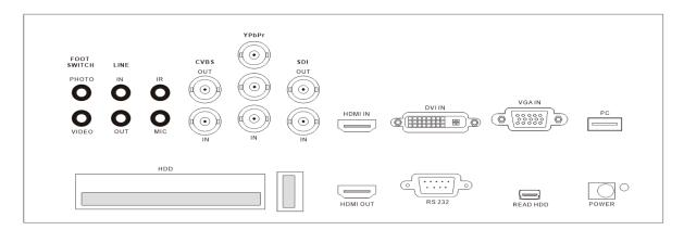
With most of video interface - SDI, DVI, VGA, HDMI, Component video and CVBS, and it detects video connection automatically. Also includes HDMI output, and loop out for SDI and CVBS.
