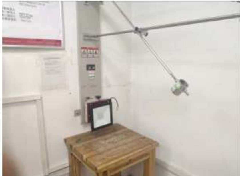
Photo 9 -- During the test of IK08
