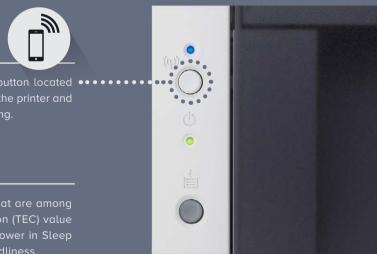
The LBP6030w comes with wireless capabilities, via the WPS button located ••••••• conveniently on the printer. Just one touch of the WPS button on the printer and router, a Wi-Fi connection is easily established for wireless printing.
