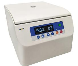
The low-speed centrifuge, popular in hospitals and blood processing centers, efficiently separates lab solutions and particles for biological sample analysis. Its adaptable design accommodates various rotor configurations and eliminates sanitary dead angles. With smooth transitions, polished surfaces, and stainless steel components, it features a LCD display for time, speed, and centrifugal force. The benchtop low speed centrifuge T5-M is equipped with the angle
