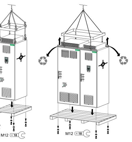
Mount the handling lugs, which are provided in a separate packaging.
