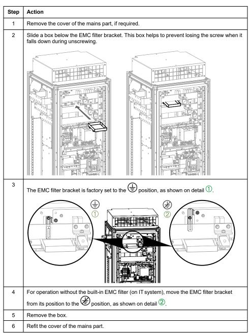
Apply the following instructions to disconnect the built-in EMC filter.
