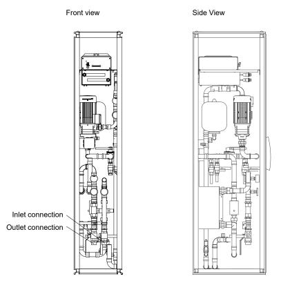
The size of the inlet and outlet fittings may be different depending on the power of the drive:
