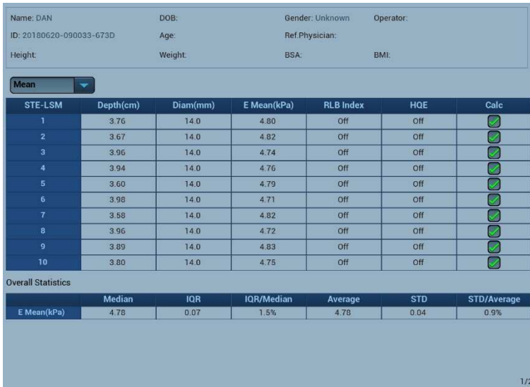
Fig. 9 The STE LSM Report displays the five acquisitions, their median values, the IQR, the IQR/M ratio, the average, the STD and the SD/Mean ratio. The median value should be considered indicative of liver stiffness. A measurement (in kPa) of good quality should have an IQR/Median \leq 30% when the median value is given in kPa and \leq 15% if the median value is given in m/s.
