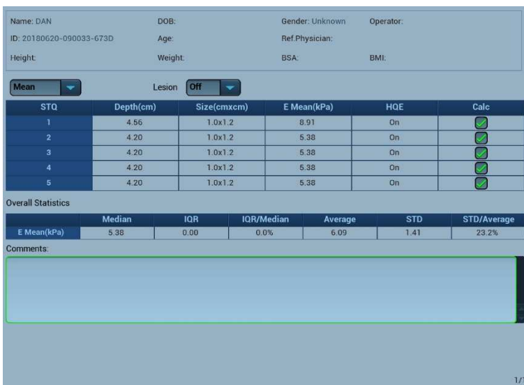
Fig. 10 Active the report box on the touch screen to auto transfer the measurement data to the table report page. The STQ LMS Report displays the IQR/M and SD/Mean ratios
