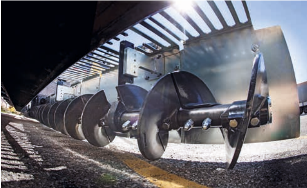
400 mm auger made of wear-resistant cast iron.
