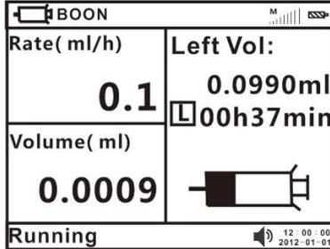
(Diagram17 Constant Flow Rate mode running interface)
