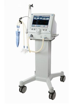
Our eVolution 3e ICU ventilators are available in a high pressure external gas source model or with an internal turbine flow generator.
