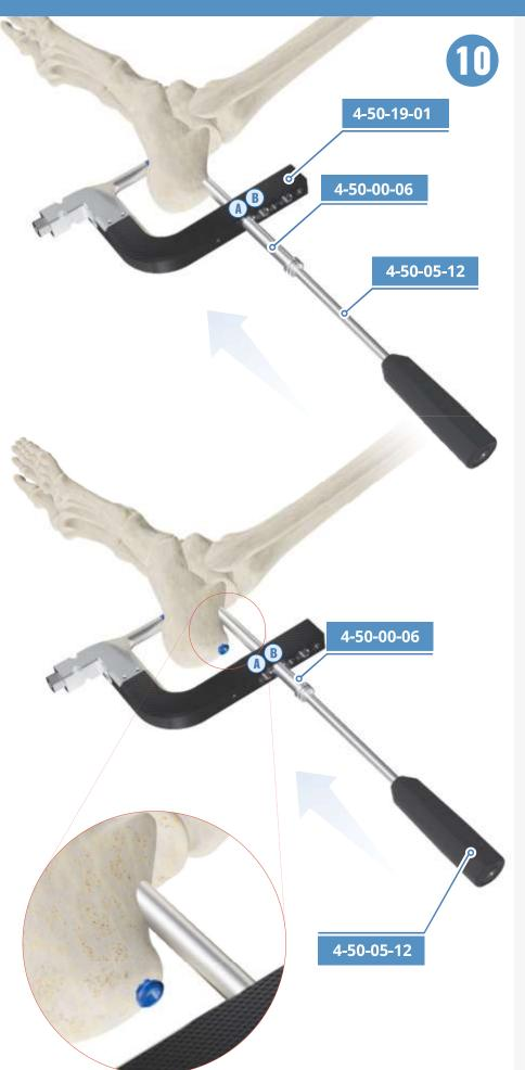
Insert the Ø 4,5 mm locking screw using screwdriver 4-50-05-12.
