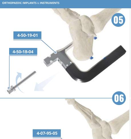
Remove M8 screw 4-50-18-04 and targeting device 4-50-19-01.
