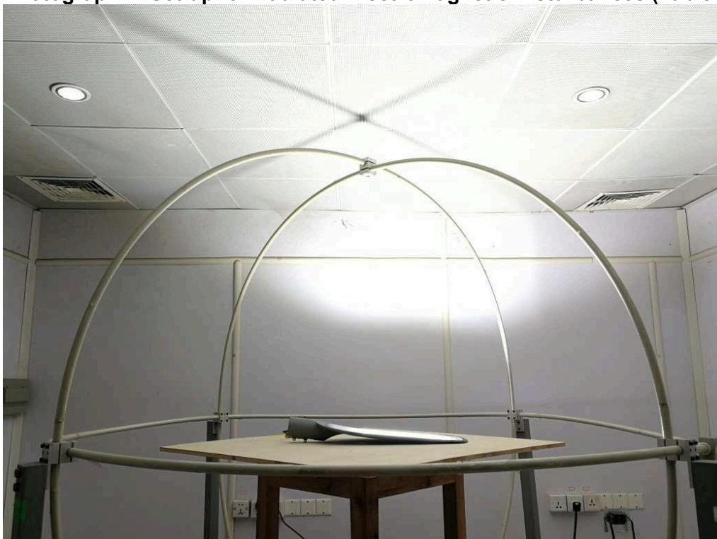
Photograph 2: Set-up for Radiated Electromagnetic Disturbances (Table 3a)
