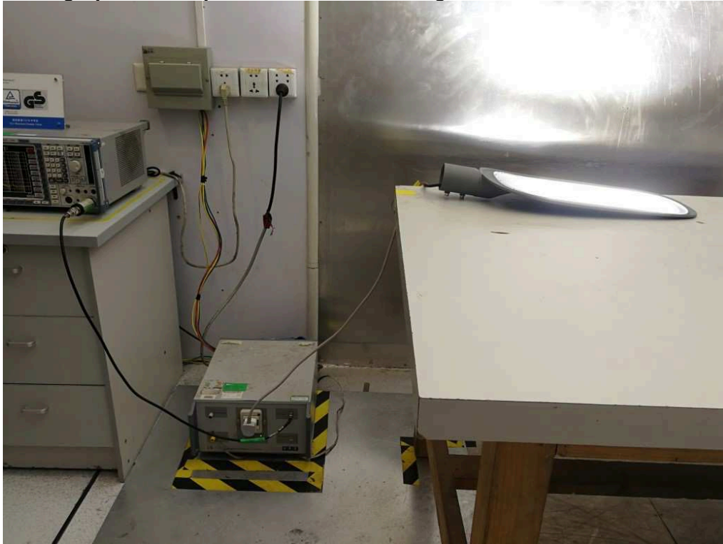
Photograph 2: Set-up for Radiated Electromagnetic Disturbances (Table 3a)
