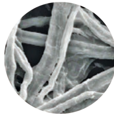
Cellulose Fiber at x500 Magnification
