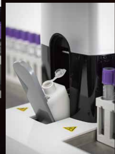
60 samples capacity autoloader with continuous loading
