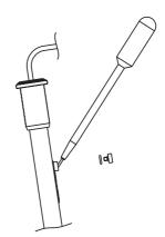
Holding the body of the electrode gently press upper cap with your thumb. This permits the fill solution to drain out of the body. Release cap and verify electrode returns to its original position. (You may need to gently assist for this to occur).
