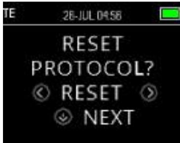
Press the **<RESET>** keys to return the selected protocol parameters to their original factory settings. Press the **∨NEXT** key to return to the Main menu.
