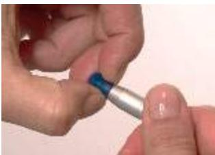
Grasp the ear tip at the base with your fingers and twist it while pulling it off the probe tube. Grasping the base of the ear tip will prevent the probe tube from being inadvertently pulled out of the probe head along with the ear tip.
