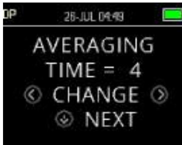
The Averaging Time refers to the test time per DP frequency. The Averaging Time will have a large impact on the time required to perform the test and, on the signal-to-noise ratio (SNR). A 2 second average for 6 frequencies would produce a test in about 18 seconds.
