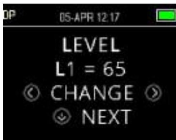
The Level L1 refers to the stimulus level of the primary tone f1 (frequency 1). The Level L2 refers to the stimulus level of the primary tone f2 (frequency 2). The intensity of the primary tones (L1, L2) may be changed to any level between 40 dB SPL and 70 dB SPL. The L1 and L2 stimulus levels can be changed in 1 dB increments by pressing the **CHANGE** keys.
