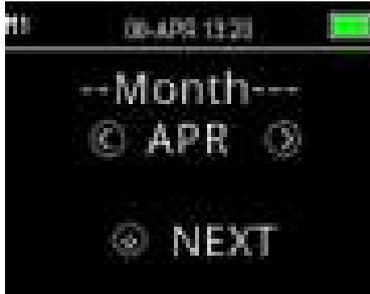
If either the date or time is incorrect, press the **CHANGE** key to access the menu to change the month. Press the **LEFT** or **RIGHT** keys to scroll forward or backward through the months.
