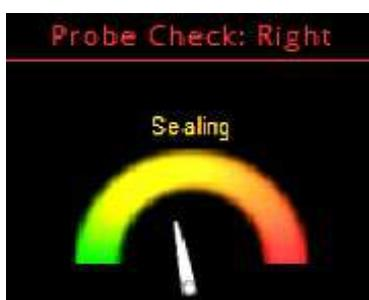
**Sealing:** The needle points to the top, yellow part of the gauge.
