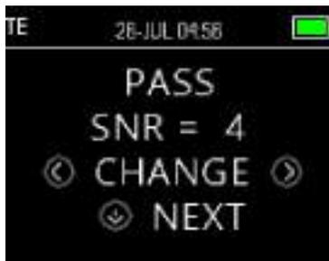
In order to provide a PASS/REFER determination for each test, the PASS SNR for all TE test bands must be set. This number refers to the number of decibels that the TEOAE signal must be above the noise to be considered as present (detected) at each frequency band. The PASS SNR can be set between 3 – 10 dB.
