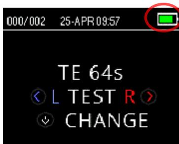
When the OtoRead™ battery's power capacity becomes low, the first indication you will see is a change of color in the battery symbol in the top right-hand corner of the display.
