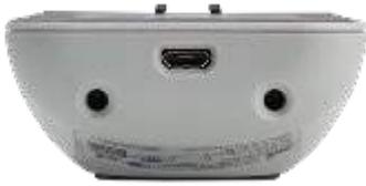
The Micro-USB port on the bottom of the instrument is the connection point for the USB used for charging via the USB cable to PC or mains.
