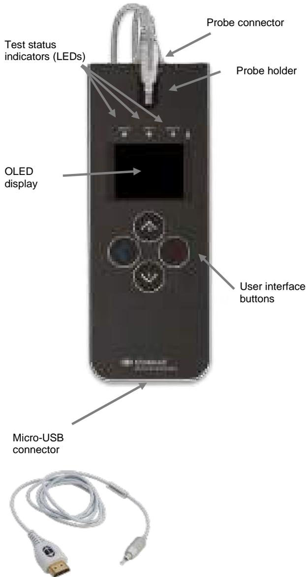
The OtoRead™ consists of the instrument, Micro-Probe, single-use ear tips, replaceable probe tubes and other accessories.
