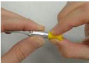
To replace the probe tube, use the ear tip to grasp the probe tube and pull the probe tube straight out of the probe body. Dispose of the used probe tube immediately to avoid confusing used tubes with new tubes.
