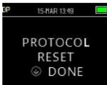
After pressing one of the **<RESET>** keys, a confirmation that the protocol was reset will be displayed. Press the **∨DONE** key to return to the Main menu.
