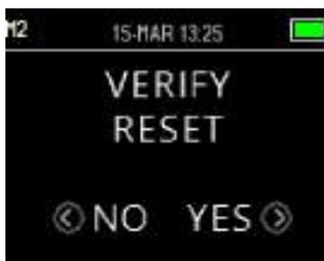
Resetting to default will un-pair the wireless device, clear the test results, and reset all system and protocol settings.
