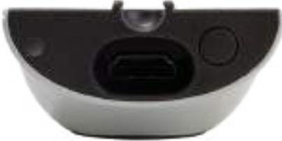
Turn off the OtoRead™ and insert the Micro-Probe plug into the socket on the top of the OtoRead™. The plug will only fit in one orientation.
