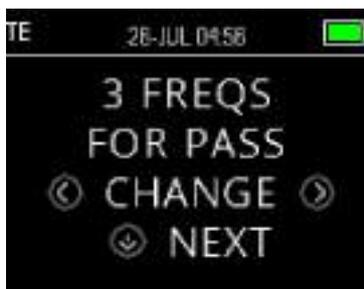
The number of frequencies (TE bands) for determining a PASS can be set from 0 to 6. If the setting is on 0, then no assessment of PASS/REFER will be made. This setting is used in conjunction with the PASS SNR and the MIN LEVEL criteria to determine the overall test outcome (PASS or REFER).
