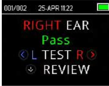
When testing is complete, the green 'READY' light is illuminated, and the display shows the test ear and test result (for screening tests).
