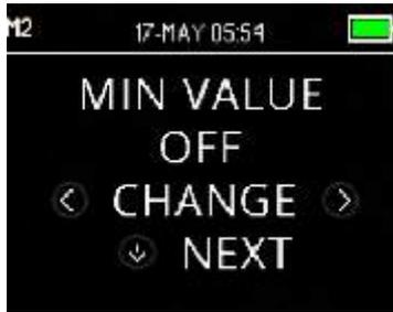
The Minimum (Amplitude) Value setting allows the user to set the unit to include minimum amplitude values in the pass/refer criterion. The OtoRead™ is set with this feature enabled when it is shipped from the factory.
