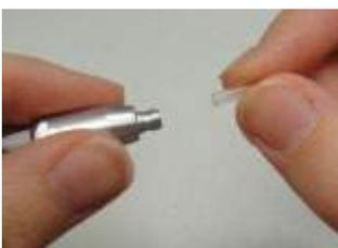
Take a new probe tube from the package and insert the tube into the probe head until it is fully seated. A properly inserted probe tube will snap securely into place when it is inserted correctly. The probe tube can also be inserted using the probe tube removal tool.
