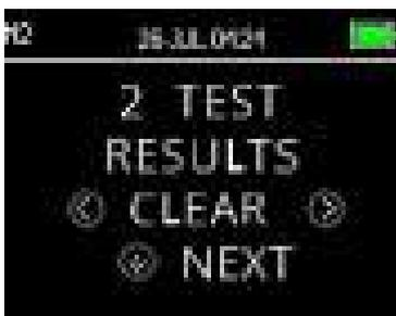
The Test Results Clear menu allows the user to clear the test results stored in the unit without printing them. Select the **< LEFT or RIGHT >** key to clear the results and select **< Yes or No >** to verify clearing or to cancel. To advance to the next menu without clearing the results, press **^ NEXT** key.
