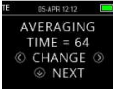
The Averaging Time for TE protocols refers to the maximum test time. The Averaging Time can have a significant impact on the signal-to-noise ratio (SNR) achieved and the final test outcome (e.g., PASS/REFER). The averaging time is independent of the probe check process.
