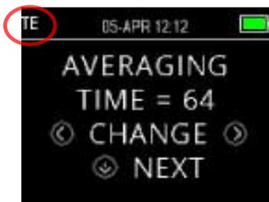
The TE protocol settings menu can be recognized by the abbreviation 'TE' in the top left corner.
