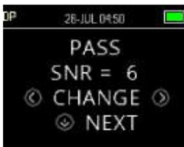
In order to provide a PASS/REFER determination for each test, the PASS SNR for all DP test frequency must be set. This number refers to the number of decibels that the DPOAE signal must be above the noise to be considered as present (detected) at each frequency. The PASS SNR can set between 3 - 10 dB.
