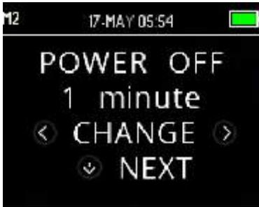
Set the Power OFF mode to define after what length of time the device will automatically shut down.
