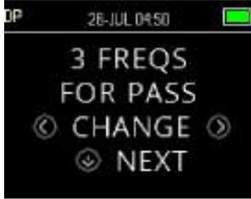
The number of frequencies required for determining a PASS can be set from 0 to 12. If the setting is on 0, then no assessment of PASS/REFER will be made. This setting is used in conjunction with the PASS SNR and MIN LEVEL criteria to determine the overall test outcome (PASS or REFER).
