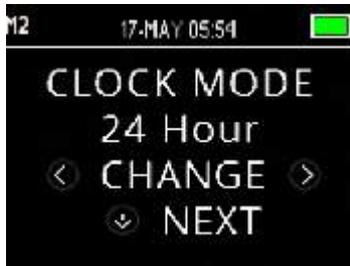
The Clock Mode menu allows the user to change the clock from a 24 hour mode to a 12 hour mode. To change the clock mode, press the **CHANGE** key. Press **NEXT** to exit this menu.
