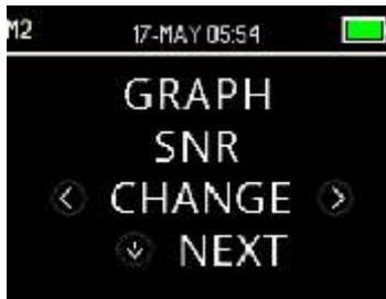
The Graph Style menu allows the user to select from two options for viewing the results. The SNR graph view shows the signal-to-ratio for each DP test frequency or TE test band. The Value graph view shows the absolute OAE and noise levels for each DP test frequency or TE test band.
