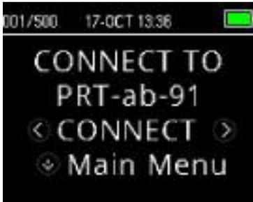
Following instructions provided with your printer, be sure the printer is on and ready for communication/printing. From the OtoRead™ instrument Main Menu, press the **^UP** key to enter the device connection screen. Press the **<LEFT** or **>RIGHT** key to connect.
