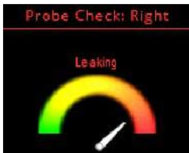
**Leaking:** The needle points to the orange, right side of the gauge.
