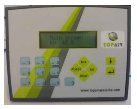
1 Press the Down arrow key ( $\downarrow$ ) on the control panel until the display reads 'RH Calibration'. Press the Enter arrow.
