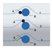
(1) Impaction occurs for relatively large particles. Due to the large inertia of a heavy particle, it does not follow the air streamline but instead travels straight ahead and collides with the glass fiber.
