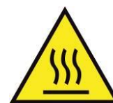
CAUTION HOT SURFACE
