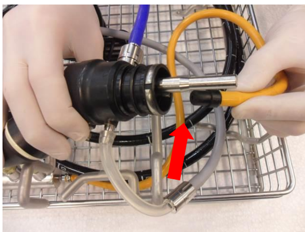
EXAMPLE OF A LEAK TEST CONECTION POINT
