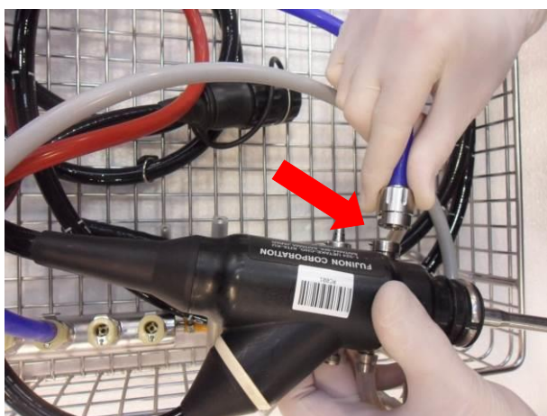
EXAMPLE OF AN AIR CONNECTION POINT
