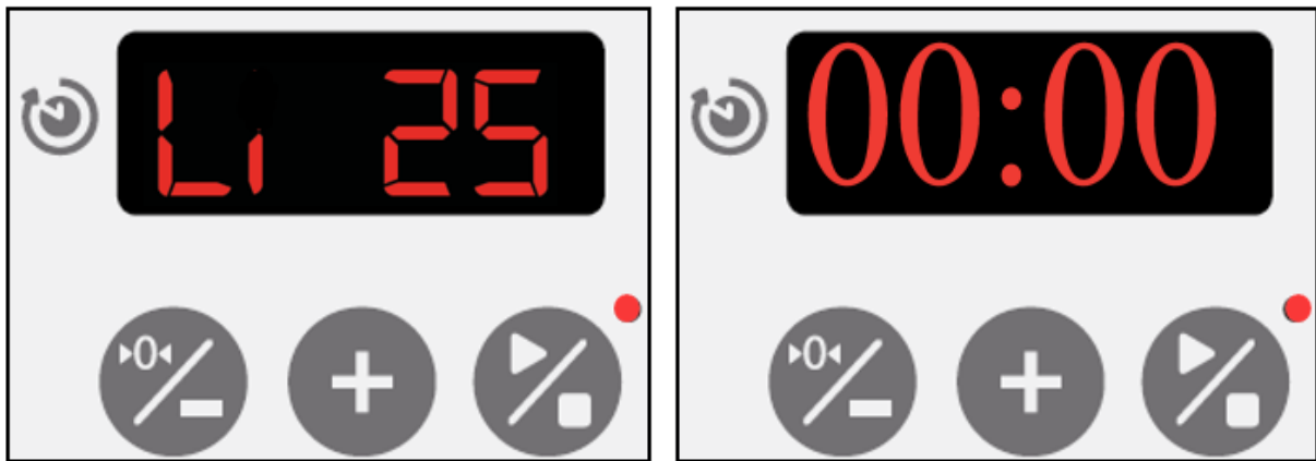
Figure 8-6. Display shows the light intensity and indicator led is ON (left). Then, display shows the phototherapy time and dots blink.
