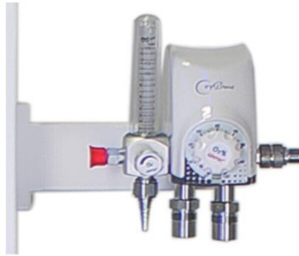
Figure 2-15. O2/air blender module
