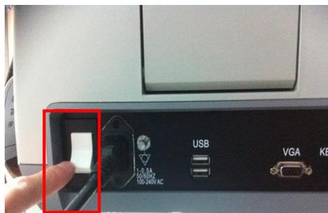
Turning off the main switch of the system
