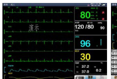
Max 8 waveform display simultaneously, max 6 leads ECG waveforms display
