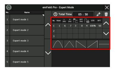
Choose the parameter to change. Wave, L (Hz), H (Hz), T1, Off, T2,, Strength, Repetition can be set in this mode by using the central control knob (6) which changes the parameter values.
