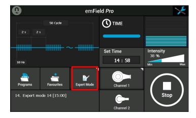
To change settings press Expert Mode on the touch screen for 2  $\sim$  3 seconds to set the parameter values.
