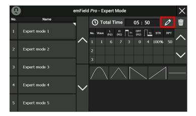
Each mode has 9 sub-modes with different parameter sets. The Expert mode operates sequentially from sub mode 1.
