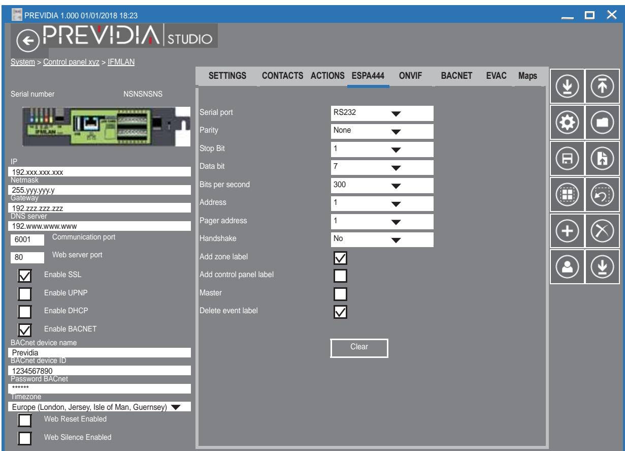
The screenshot shows the Previdia Studio software interface for configuring the IFMLAN module. The left sidebar shows the system path: System > Control panel xyz > IFMLAN. The main window has tabs for SETTINGS, CONTACTS, ACTIONS, ESPA444, ONVIF, BACNET, EVAC, and Maps. The ESPA444 tab is selected. On the left, there is a preview image of the IFMLAN module and several configuration fields:
